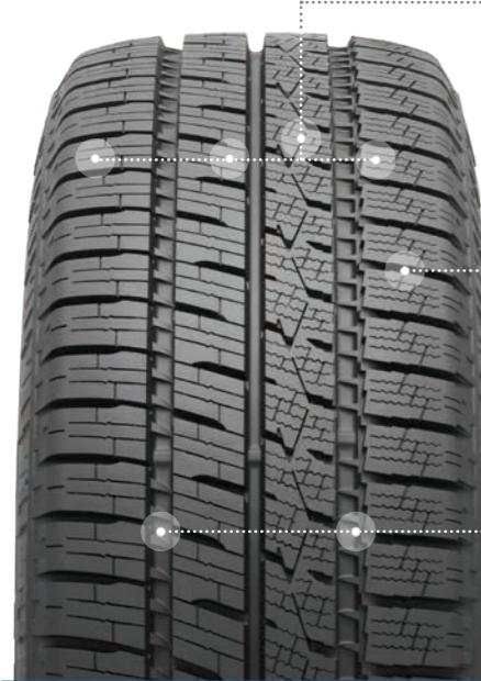
The asymmetrical profile design uses fine sipes within the tread blocks to rapidly channel water away and provide excellent traction.
