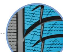
Wide shoulder blocks offer an extensive contact area, delivering excellent road grip and enhanced braking performance.
