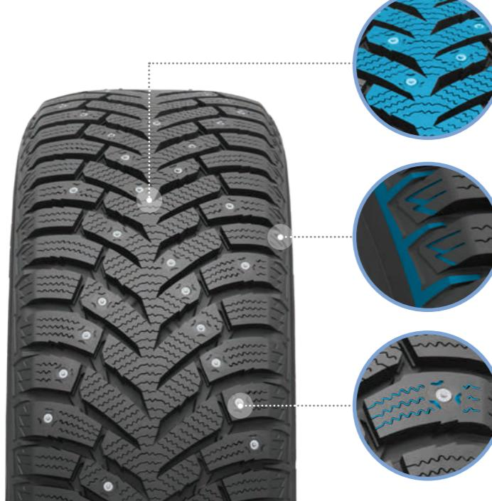
The tree shaped centre tread block improves traction and braking performance on ice and snow.
