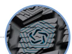
The 360° sipes, which give the tread block a special honeycomb structure with small, transverse grooves, improve grip on snow and icy roads.
