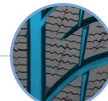
Two wide circumferential tread grooves quickly drain the water from the small tread block sipes, thereby improving grip on wet and wintry roads.
