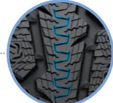
A wave-shaped sipe runs along the centre tread blocks channeling water and improves road contact in winter conditions.
