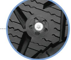
The tire is designed with a V-shaped directional tread pattern that efficiently evacuates water. Additionally, spikes in the tread blocks provide increased grip and traction.
