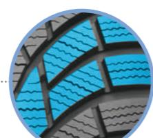
The tread blocks feature sipes that run in various directions, allowing a quick water drainage and maintaining optimal road contact.
